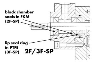
Standard inlet pressure p1: 7 bar (in certain special solutions up to 50 bar!) Before start-up the block chamber must be filled with fluid. Beinlich recommends using Mesamoll<sup>®</sup> oil or another inert medium which does not react with the pumped fluid and which is environmentally inert should it leak. The block chamber is formed by the seal housing or by attaching a drip-feed lubricator.
