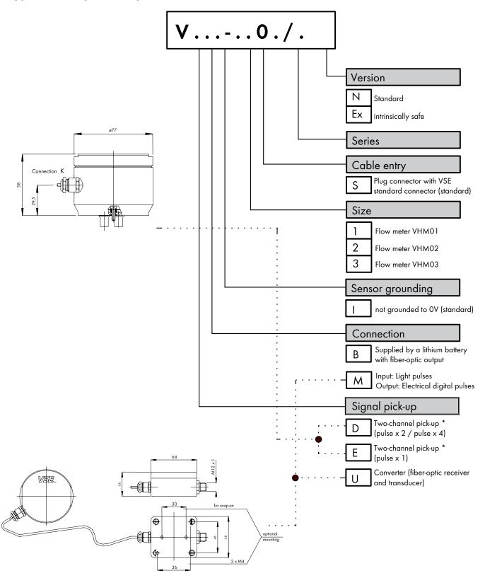
\* With the VDB series... (fiber-optic output), the signal can only be doubled (pulse x 2)
