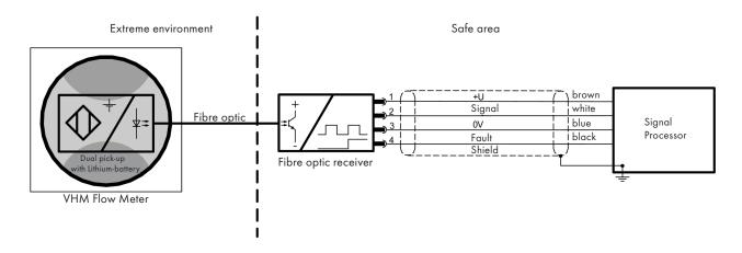
Figure 3: Wiring diagram for the measuring system
