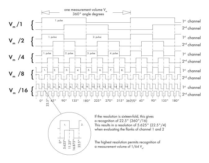
Fig. 3: Interpolation of the volume measurement  $V_m$
