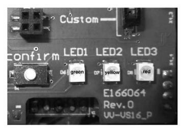
Fig. 5: Indicating LEDs of the peripheral board
