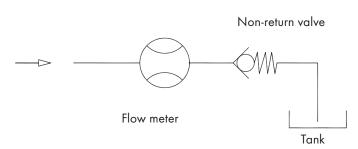
Fig. 1: Flow meter installation with non-return valve
